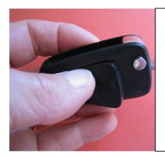
Place a new silicone pad over top part of your remote. Use rolling motion when positioning pad in grooves and press firmly till pad "engages" with hard shell all around edges and in the middle. If pad is not sitting in level with the shell you can use finger nail to push it deeper in the groove.
